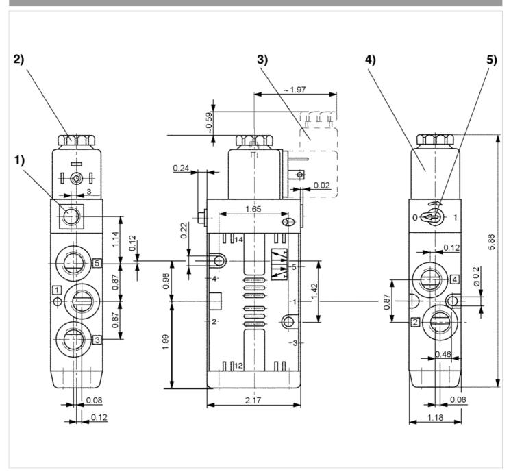
1) Only with separate pilot control G 1/8 2) After removal of cap M5 internal thread 3) Valve plug connector4) Coil can be plugged at 45° intervals 5) Manual override
